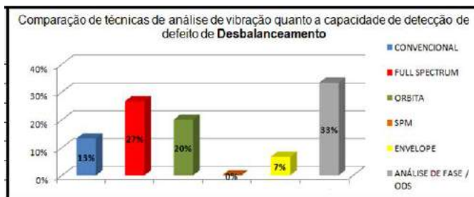
Figure 3.19: Final Graph of techniques evaluation for unbalance detection.
